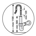
Fit the drainage hose of your machine to the drainage pipe without bending.
