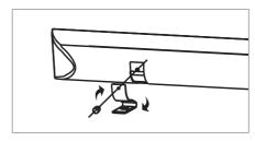
5 Place the included washer and then the snap ring onto the fixing bolt and reattach the unit base through the second drill hole.
