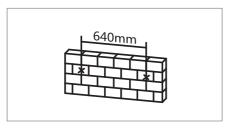
2 Drill the holes (8 mm Ø) in the wall and insert the plugs included.
