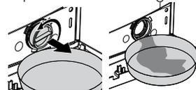
Place a large container in front of the filter to catch water from the filter. Loosen pump filter (anticlockwise) until water starts to flow. Fill the flowing water into the container you have placed in front of the filter. Always keep a piece of cloth handy to absorb any spilled water. When the water inside the machine is finished, take out the filter completely by turning it.
