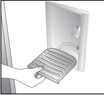
Make sure that the parts removed (if any) during cleaning are properly attached to their original places. Otherwise, water leakage may occur.
