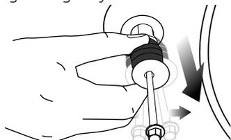
3. Attach the plastic covers supplied in the User Manual bag into the holes on the rear panel.
