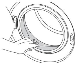
If the holes on the bellow shown in the figure are blocked, open the holes using a toothpick.
