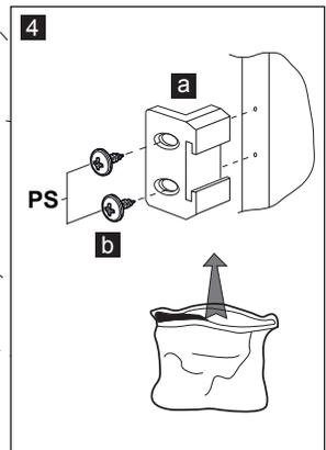
**Note:** Installation step for 2, screws for connecting top plastic part should not be screwed very hard, because of moving the plastic part easily left or right side.
