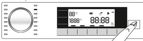
If the water level in the machine is not suitable when you press **Start / Pause** button, the loading door symbol remain lit on the display.
