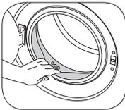
After every washing make sure that no foreign substance is left in the drum. If the holes on the bellow shown in the figure is blocked, open the holes using a toothpick.
