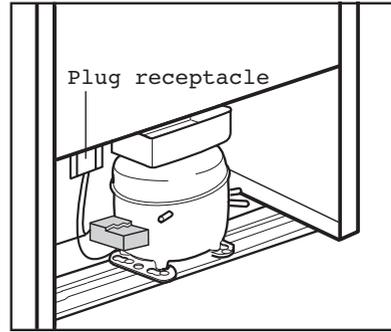
case of transportation, ensure you locate the plug in the receptacle provided to avoid transit damage.
