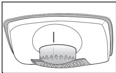
Operating temperatures are controlled by the setting knob (see diagram) located on the ceiling of fridge compartment. Settings may be made from min, 1 ... 6, max, max being the coldest position.
