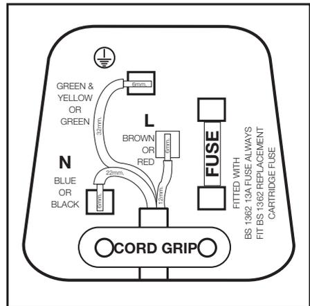
**3.** Connect the brown (Live) wire to the terminal in the plug marked 'L' or coloured red.
