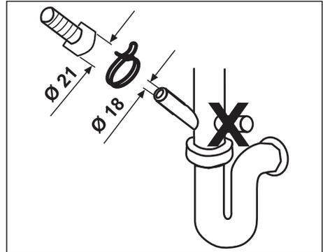
A discharge hose longer than 4 meters causes dirty washing. Attach the water discharge hose to the drainpipe without bending it. Tightly fix the water discharge hose to the drainpipe in order to prevent any dislocation of the water discharge hose during operation of the product.
