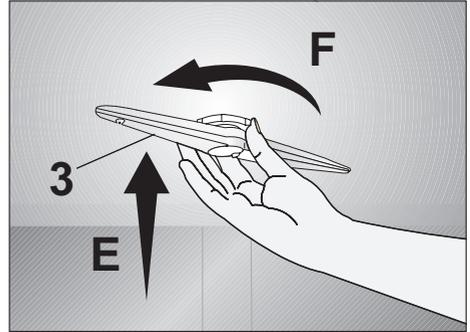
To remove the impeller, slightly (E) push it upwards and then turn clockwise (F).
