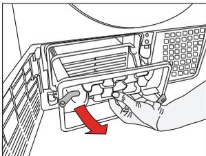
4. Clean the condenser by applying pressurized water with a shower armature and wait until the water drains.
