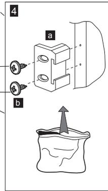
**Note:** Installation step for 2, screws for connecting top plastic part should not be screwed very hard, because of moving the plastic part easily left or right side.
