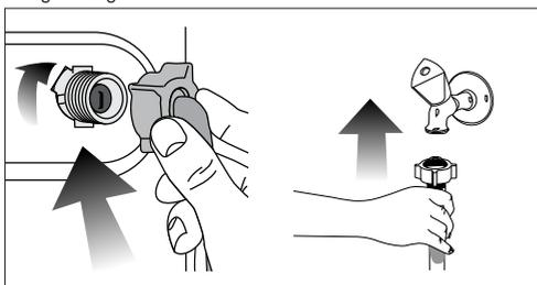
2. Open the taps completely after making the hose connection to check for water leaks at the connection points. If any leaks occur, turn off the tap and remove the nut. Retighten the nut carefully after checking the seal. To prevent water leakages and damages caused by them, keep the taps closed when the machine is not in use.
