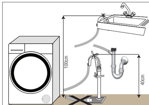
1. Tighten all hose nuts by hand. Never use a tool when tightening the nuts.
