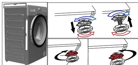
1. Loosen the lock nuts on the feet by hand.
