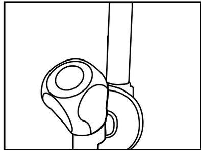
4. Attach the water hose extending from the top of the filter to the product's water connection adaptor, (see 3.6.)
