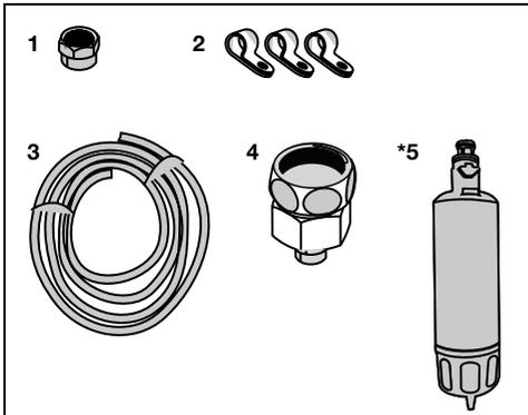
1. Connector (1 piece): Used to attach the water hose to the rear of the product.
