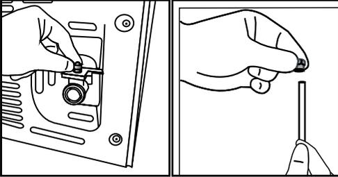
2. Push the water hose down tightly and connect to the hose nozzle adaptor.
