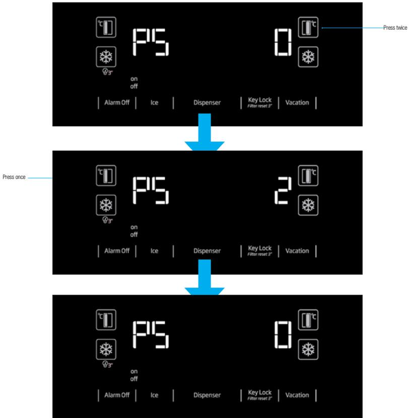
“Upon seeing PS 0 screen, de-energise the refrigerator and energise it again. This way, the filter counter will be activated. The filter warning LED will be active on the display in 130 days. After replacing the filter with a new one, press the Key Lock button for 3 seconds to make the filter counter to count down from 130 days.
