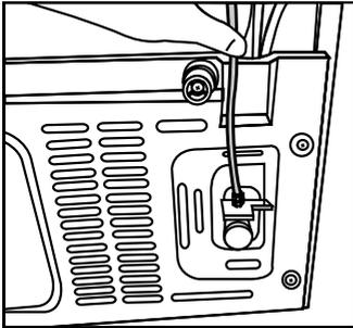
3. Tighten the connector manually to fix on the hose nozzle adaptor. You may also tighten the connector using a pipe wrench or pliers.
