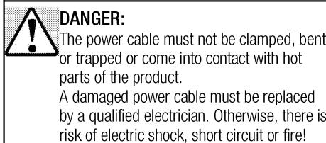
The mains supply data must correspond to the data specified on the type label of the product. The rating plate is either seen when the door or the lower cover is opened or it is located at the rear wall of the unit depending on the unit type. Power cable of your product must comply with the values in "Technical specifications" table.
