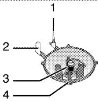
1 Flame failure device (model dependant)
