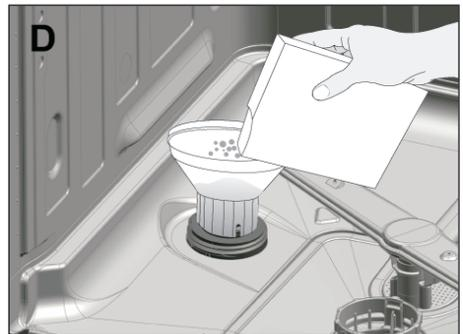
5. If you will not start a washing programme immediately after adding the salt, run the machine empty in the shortest programme to dissolve and wash away the scattered salt in the machine.
