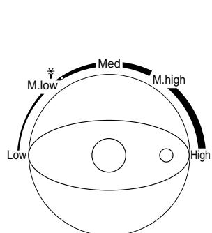
Turn Power Control knob to correct required power level.
