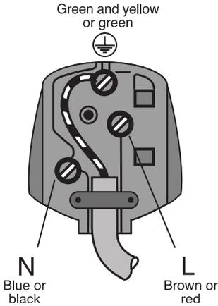
As the colours of the wires in the mains lead of this appliance may not correspond with the coloured markings identifying the terminals on your plug, proceed as follows:
