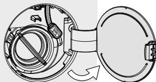
a) Open the pump filter cap.
