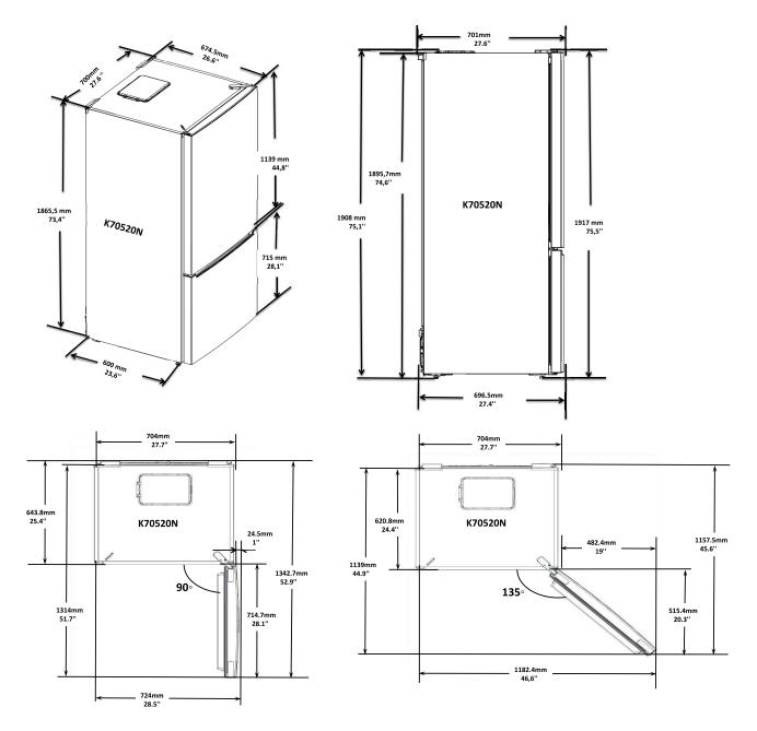
WARNING: When installing the appliance next to a wall, a distance on the hinge side of 1 inches (24.5 mm) minimum is required between the appliance and the wall to allow for the door projection when the door is open.
